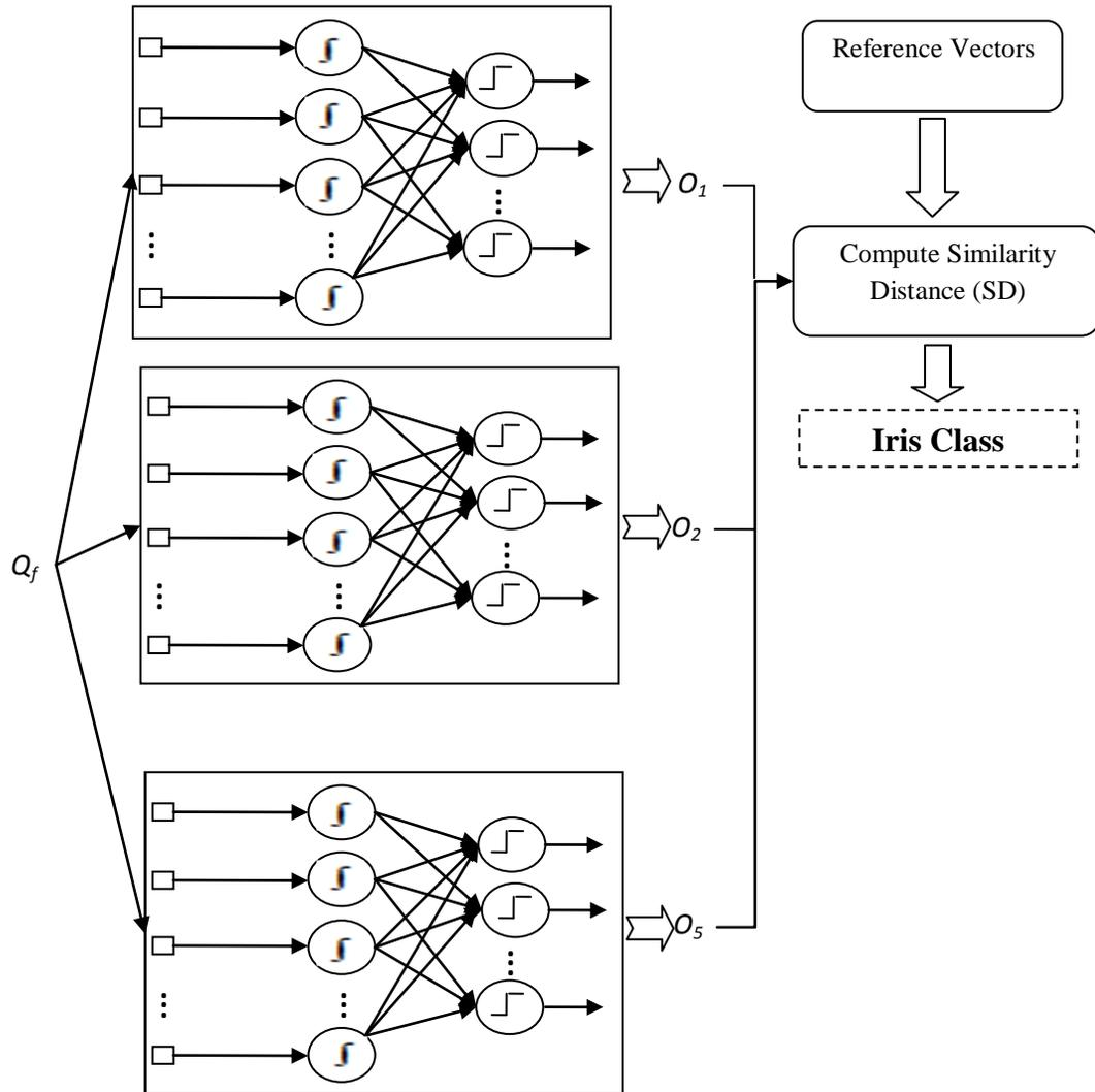
Figure 5.3 Architecture of each module of the neural network
