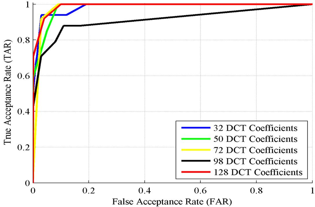
Figure 5.6 ROC curve of the optimal neural network with 32, 50, 72, 98 and 128 DCT coefficients
