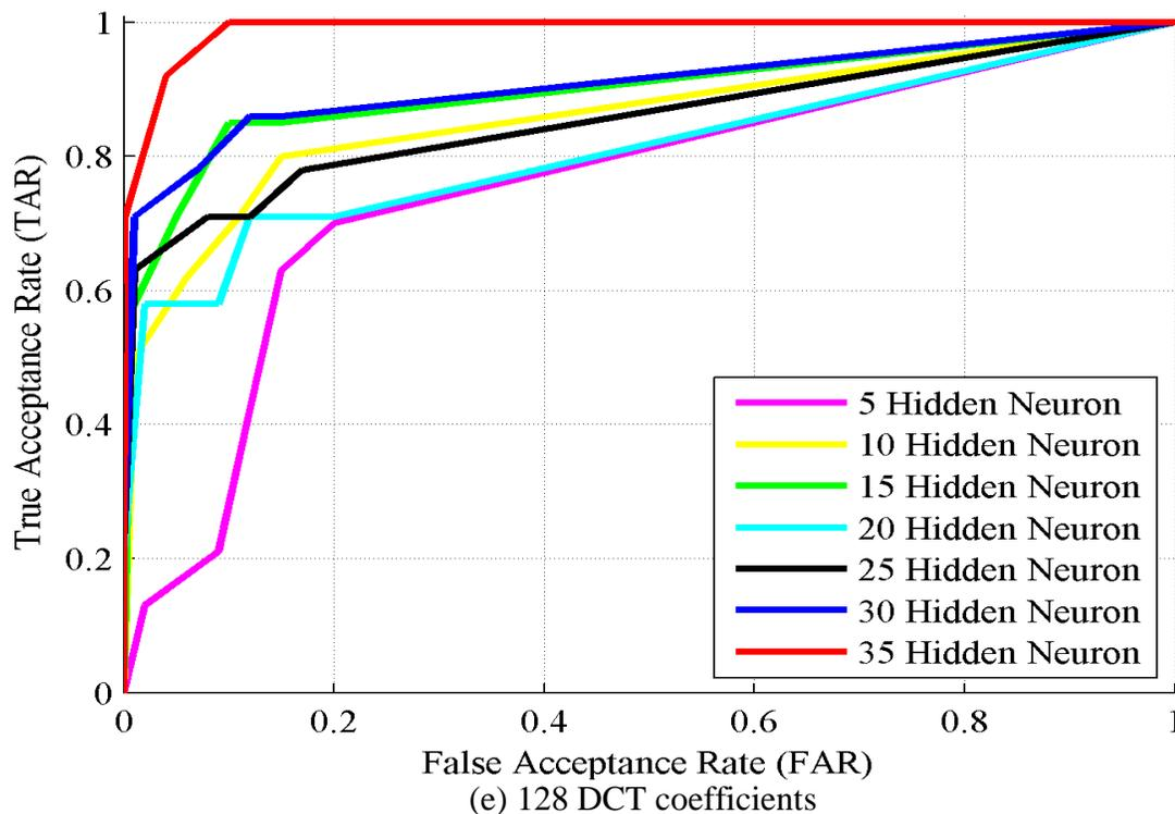
Figure 5.4 Network ROC curve on testing dataset with different DCT coefficients by varying the number of hidden neuron over MMU2 iris dataset (Continued...)
