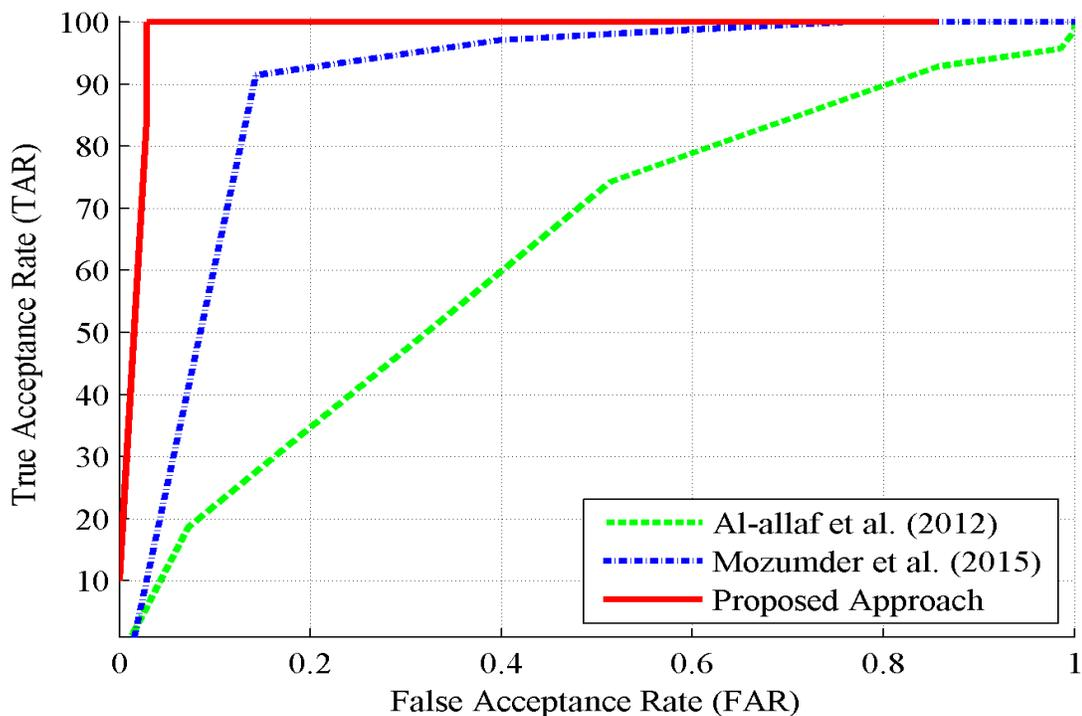
Figure 5.8 ROC curve of the proposed recognition approach, Al-allaf *et al.* (2012) approach and Mozumder *et al.* (2015) approach on verification mode over the MMU2 iris dataset
